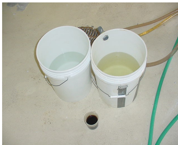
Figure 2: MIEX ® treated water (L) compared to the raw water (R). The small beaker contains brine after regeneration of loaded resin
