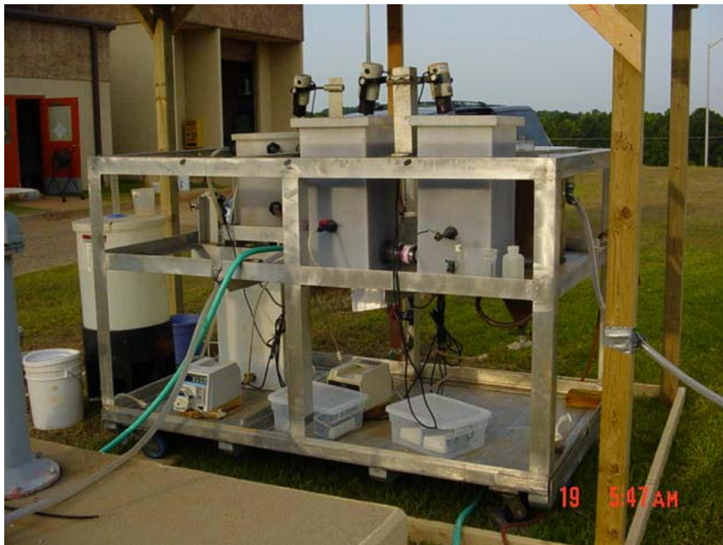
Figure 3: MIEX ® Pilot Plant at the Mims WTP
