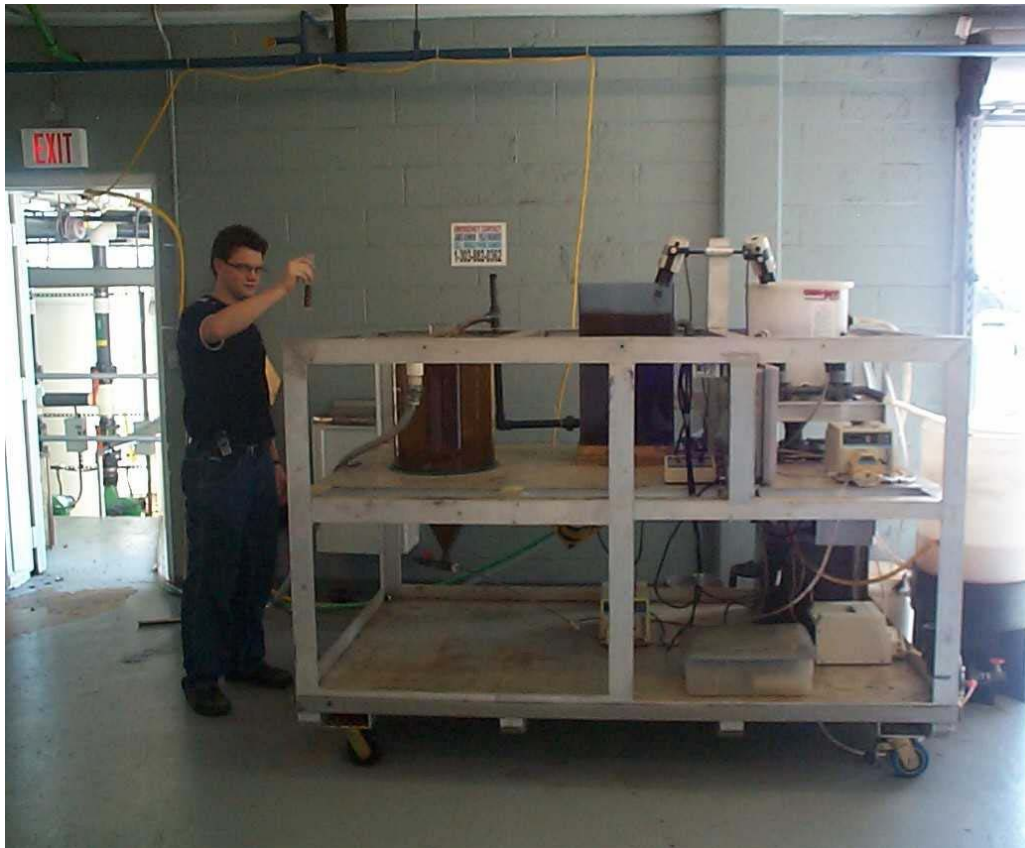
Figure 2: MIEX ® Pilot Plant at Olga WTP
