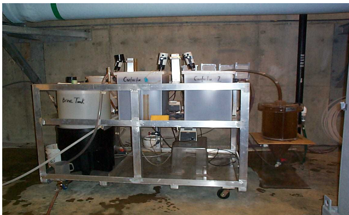
Figure 1: MIEX ® Pilot Plant at Northwest River WTP
