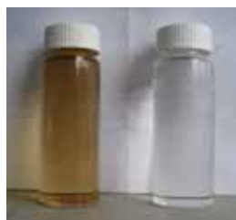
Figure 1: Biologically treated pulp mill effluent (Left) & biologically treated effluent after MIEX® Treatment (Right)
