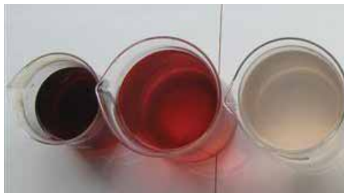
Figure 2: Dyehouse effluent comparison. Raw Effluent (Left), Existing coagulation (Center), MIEX® Treatment & coagulation (Right)
