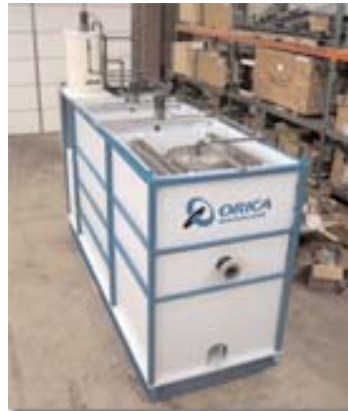
50 gpm MAGNAPAK ™ System prior to installation at Big Elk Meadows
