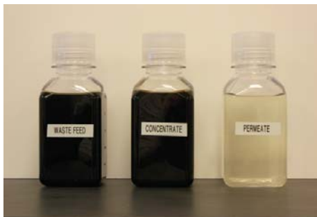
Figure 7: Initial Feed (Left), Concentrate (middle) and Permeate (Right)
