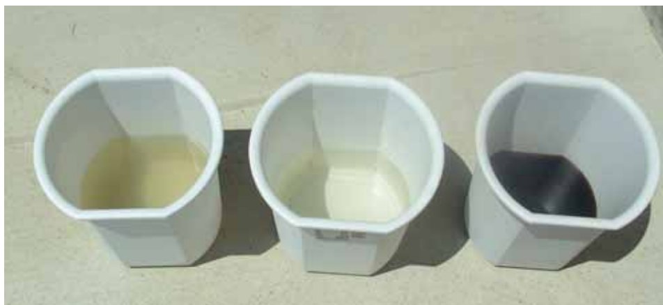
Figure 2: Portsmouth settled raw water (left), MIEX® Treated water (center) and TOC/DOC removed from water (right)
